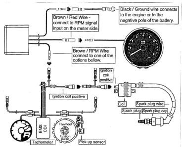
When connecting the RPM wire, follow the instruction above. If you connect the red & brown wires in parallel this may damage the instrument.
