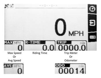
Press the **UP** button to alternate between **Maximum Speed** and **Average Speed**.
