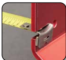
Magnets hold tapes in place during use.
