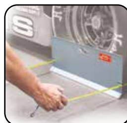
Magnets hold tapes in place during use.
