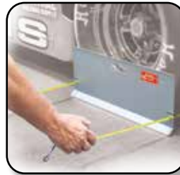
Magnets hold tapes in place during use.
