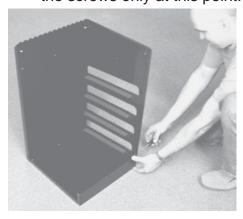
3) Position the second tray about 2" from the top, align the holes & start the screws
