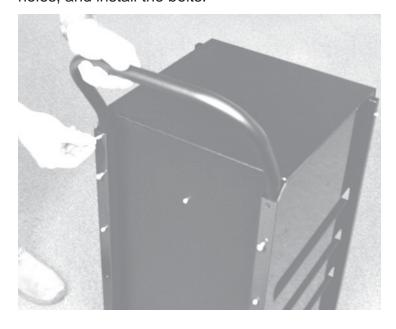
8) Line up mounting holes and start screws.
