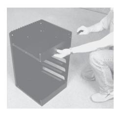
4) Put the lid in place by aligning the hinge end with the back. Push the hinge pin in from the side. Be careful not to bend the pin.
