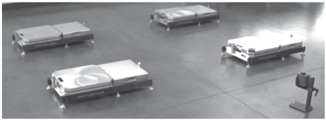
**Step 1:** Set up the scale pads or roll-offs using your car's wheelbase and track width so that the pads will be centered on the tires.
