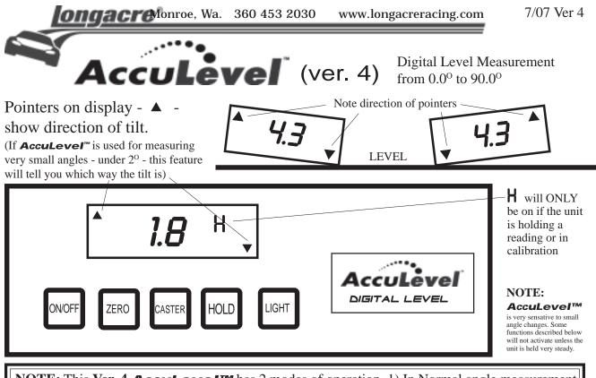
**<u>NOTE</u>:** This **Ver. 4** *AccuLevel*<sup>TM</sup> has 2 modes of operation. 1) In Normal angle measurement mode the display is steady. 2) In Caster Mode the display flashes (and will not measure absolute angles). Push CASTER button to exit Caster mode and go back to Normal angle measurement.
