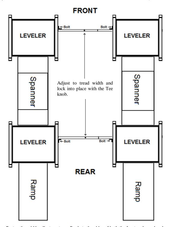
Fasten the width adjustment arm firmly to the sides of both the front and rear levelers.
