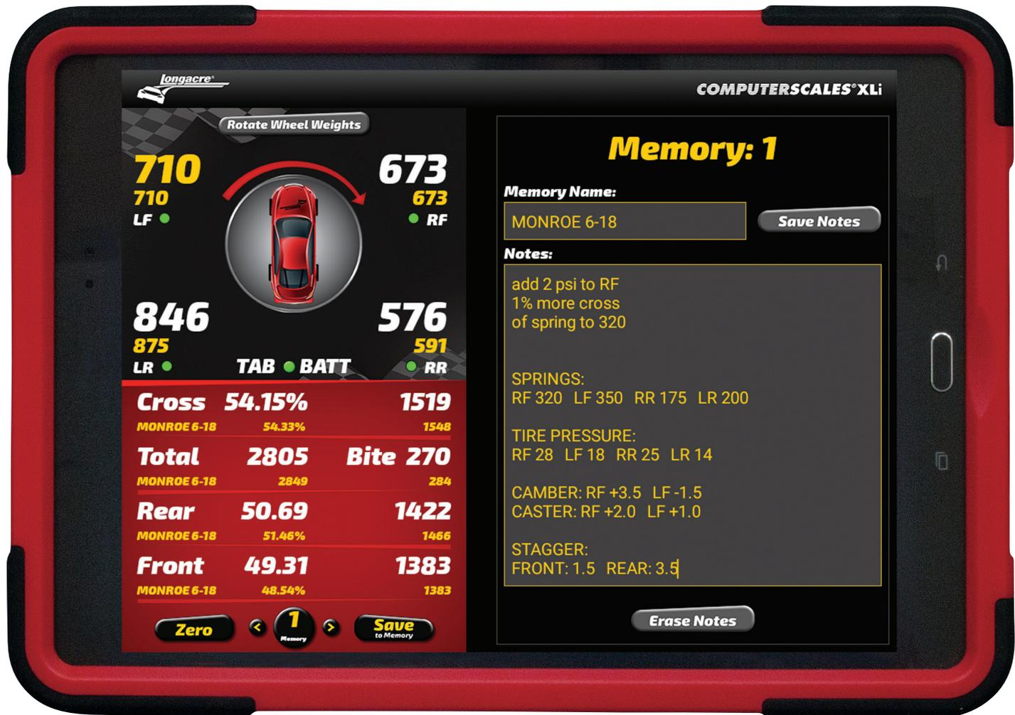
**ROTATE WHEEL WEIGHTS ON DISPLAY:** Tap the Rotate Wheel Weights button. Weights and car icon rotate clockwise in 90° increments. This is helpful if you are standing at the front or the side of the car. The wheel weights are oriented to where you are standing.
