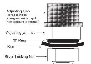
Use the low pressure springs to convert TIRELIEFS to 3 - 15 psi pressure range. Simply loosen the thin jam nut, unscrew the cap and replace the spring. Reassemble and adjust.
