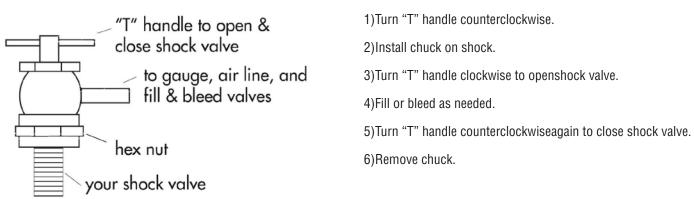
These Shock Inflators include a special chuck that allows you to add pressure or bleed, then remove the chuck from shock without losing any pressure in the shock. The "T" handle on the top opens and closes the shock valve separately.
