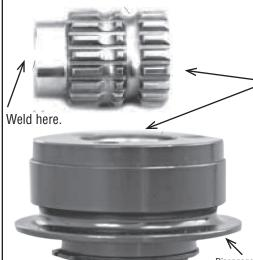
This steering shaft spline has an second safety engagement groove.
