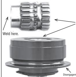
This steering shaft spline has an second safety engagement groove.
