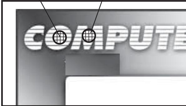
1) Turn on control box. There is a "hidden" button at the upper left of the face. It is hidden because it is rarely used and allows the user to get into *System Test* mode. There are 2 possible locations for this unmarked hidden button, depending on age. See at left. If you push in one location and get no response or hear no beep try the other. When you push in the correct location you will hear a beep.
