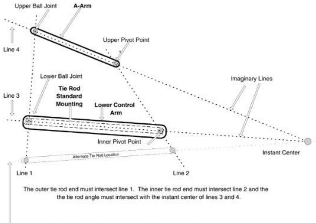
The outer tie rod end must intersect line 1. The inner tie rod end must intersect line 2 and the tie rod angle must intersect with the instant center of lines 3 and 4.
